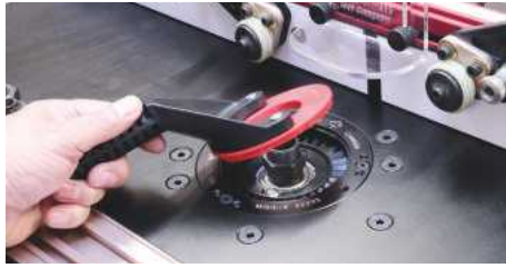
▲ Reducing inserts are quickly secured or changed with the Tab-Loc wrench
